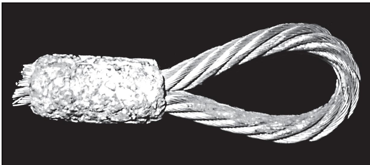
Fig. 51: Manchon aluminium corrodé
