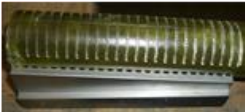
Figure 45: Imprints on the resin sleeve from the wedge faces after loading in the socket.
