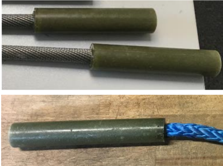
Figure 44: Wire (top) and fibre (bottom) ropes with cylindrical resin sleeve ready for mounting the in wedge socket.
