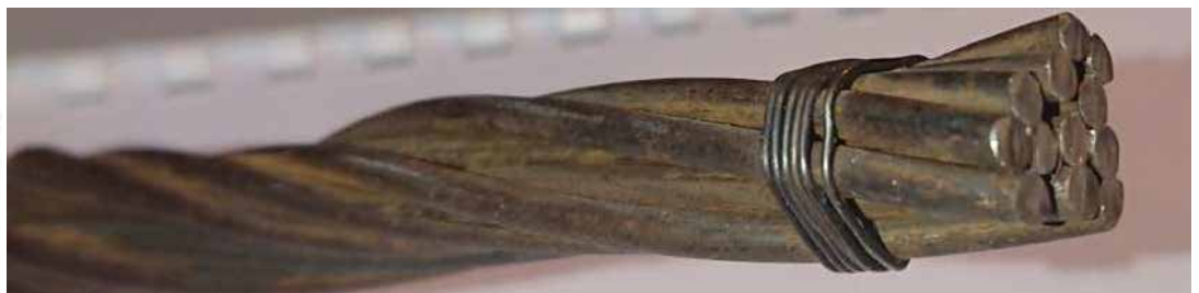
Multi strand rope (Julius Albert) – theoretical section (left), and replica by Roland Verreet (right).
