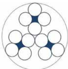
Multi strand rope (Julius Albert) – theoretical section (left), and replica by Roland Verreet (right).
