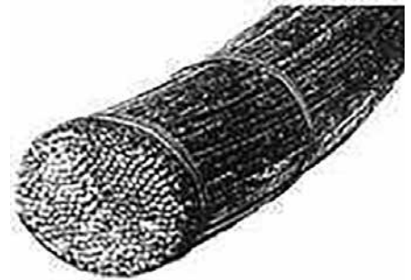
Rope with parallel wires (Marc Seguin).
