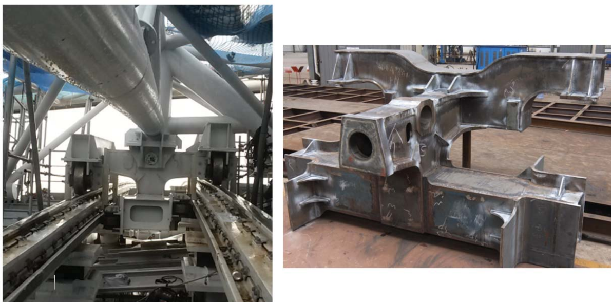
Figure 11: Bogie for RWT3 – on site and during production.
