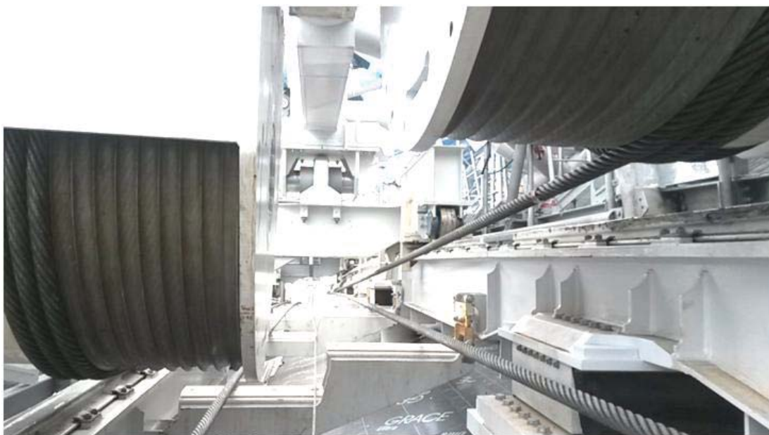
Figure 25a: Open position – Dead wraps on the drum.
