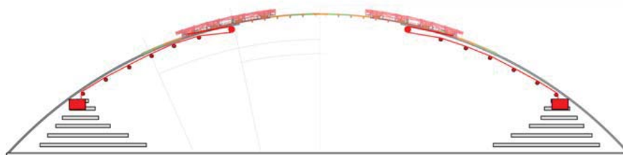
Figure 17-b: Winch rooms on the top of the concrete structure
