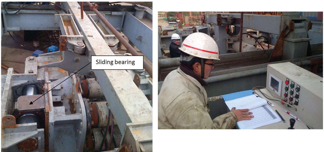
Figure 13: Sliding bearing – test stand.
