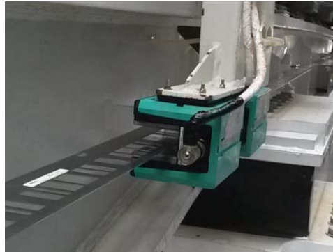
Figure 21: Linear encoder – position measurement.
