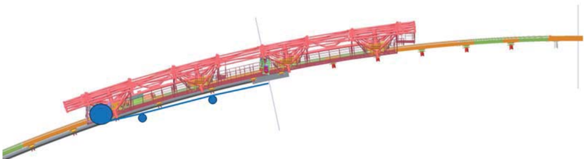
Figure 18-b: Winch on the rear side of the moving roof
