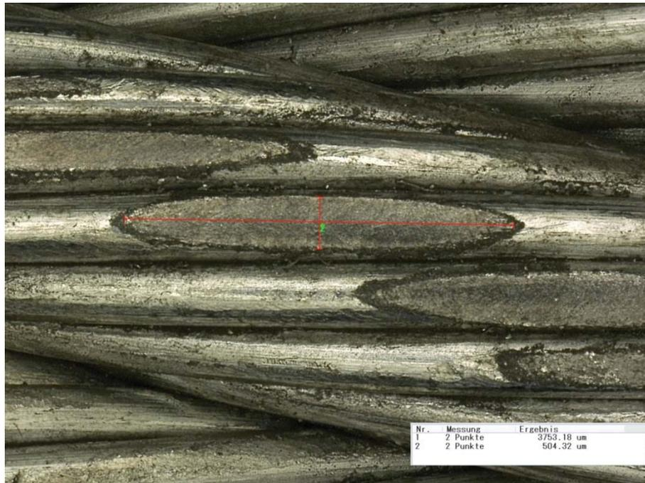
**Figure 13:** Wear ellipse of a steel wire rope tested without lubricant after 20% of the number of bending cycles to failure.
