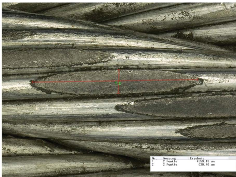
**Figure 14:** Wear ellipse of a steel wire rope tested without lubricant after 40% of the number of bending cycles to failure.
