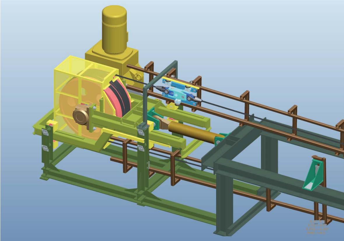
Figure 7: Drive unit with double drum and rope tensioning cylinder.
