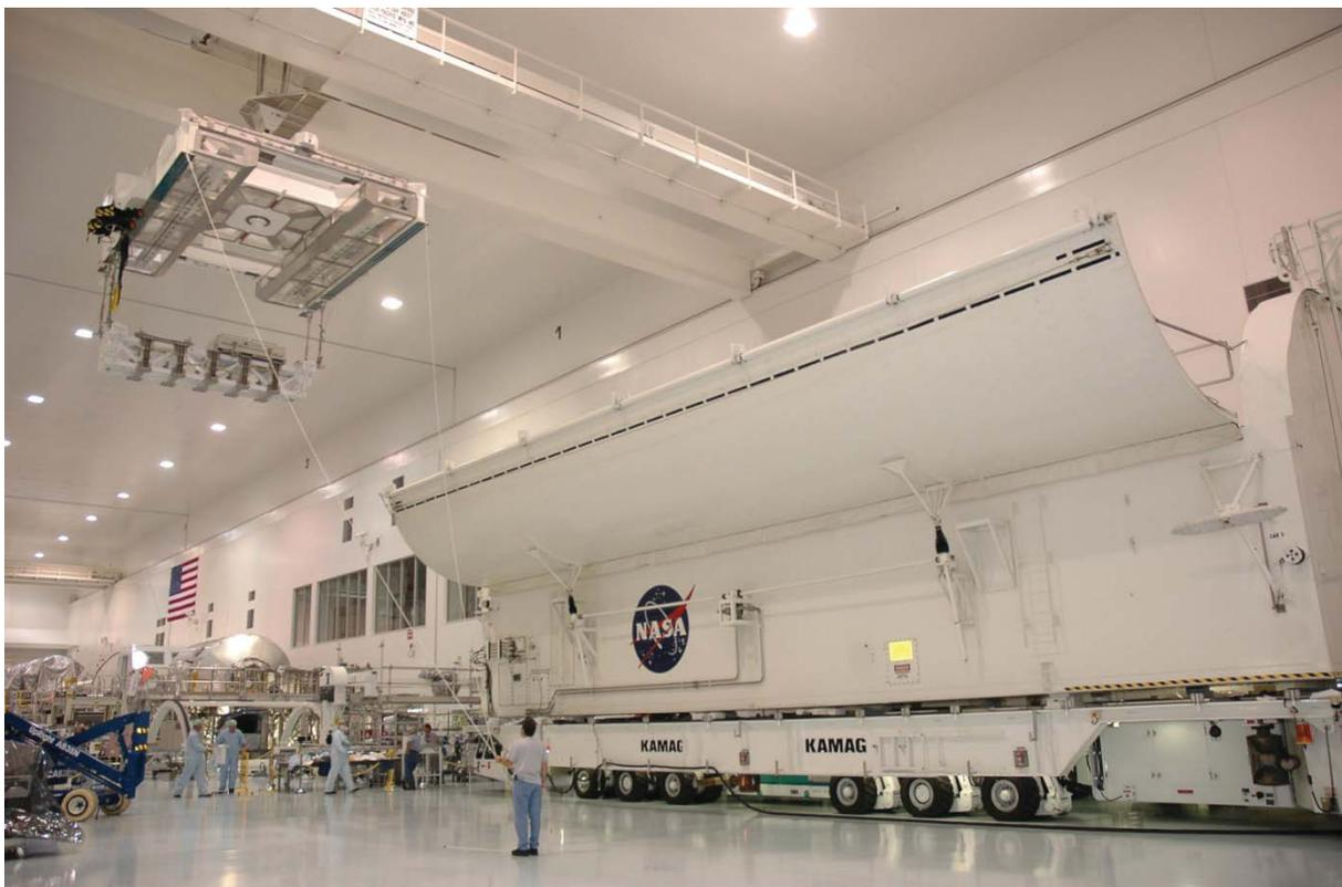
**Figure 10:** The 30t overhead crane in the NASA Space Station facility.
