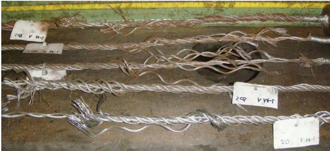
**Figure 11:** Rope sections which had been subjected to 0% (bottom), 20%, 40%, 60% and 80% (top) of the bending cycles to failure after break testing.
