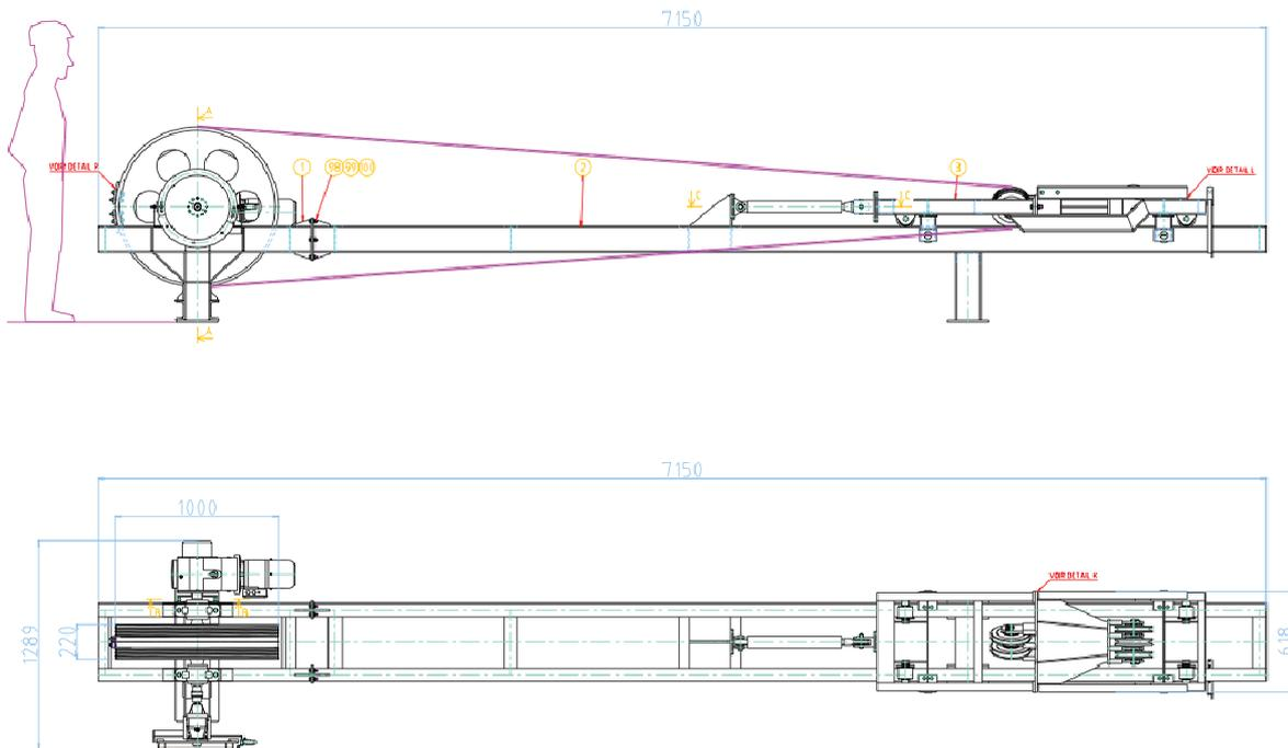
**Figure 5:** Small bending fatigue machine (rope diameter up to 10mm).
