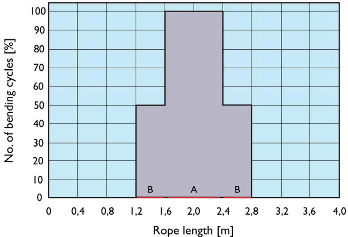
**Figure 2:** Bending cycle distribution in a conventional fatigue machine.
