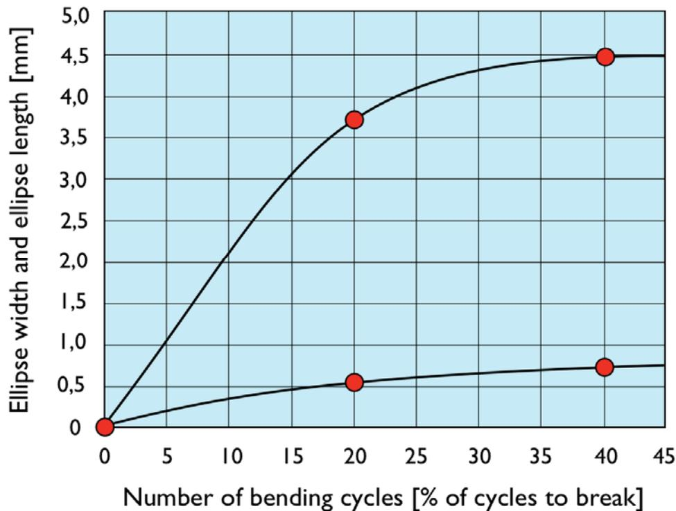
**Figure 15:** Evolution of the wear ellipse length (top curve) and width (bottom curve) over the rope life.
