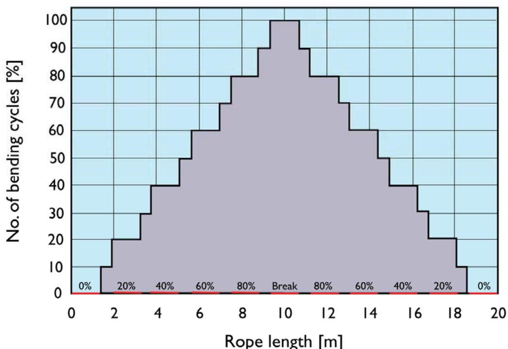
Figure 9: Distribution of bending cycles along the length of the test rope.
