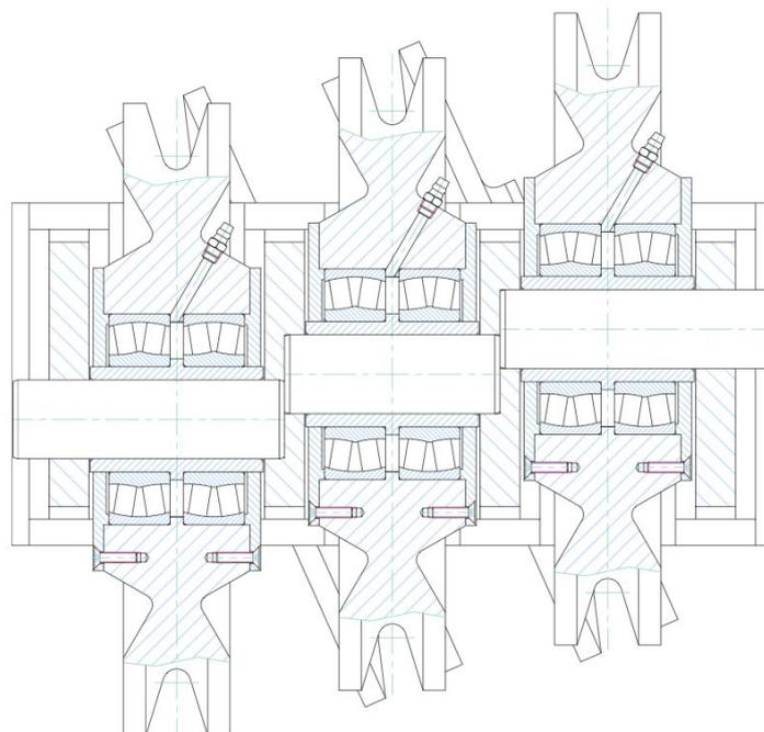
Figure 4b: Sheave arrangement of the test machine.
