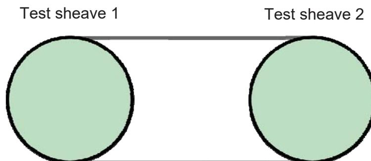
**Figure 3:** Conventional bending fatigue machine with two test sheaves and a closed rope loop.
