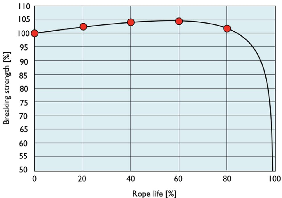
**Figure 12:** Evolution of the breaking strength of a non-lubricated steel wire rope. At 80% of the number of cycles to failure the rope still has a higher breaking strength than when it was new.
