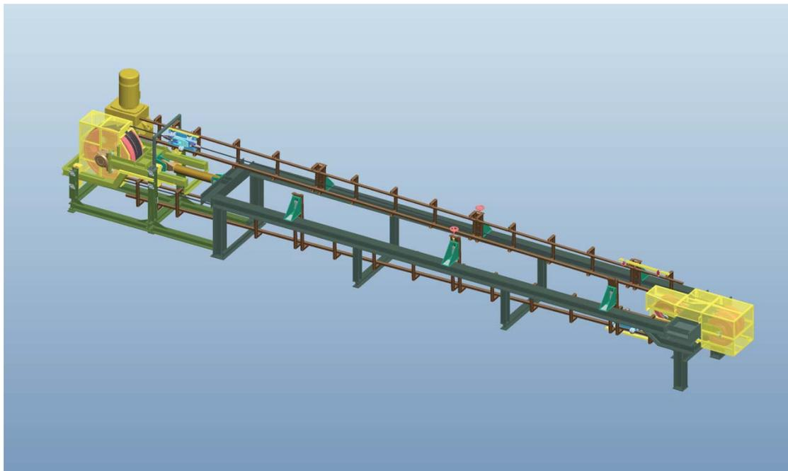
**Figure 6:** Test machine for ropes up to 30 mm diameter.
