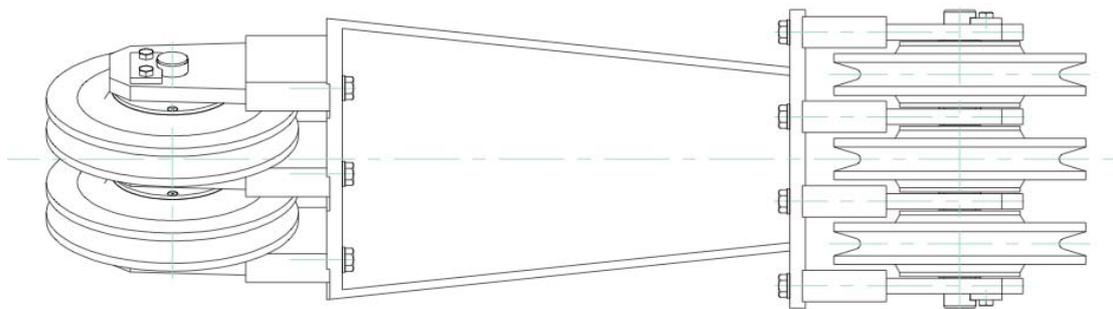
Figure 4a: Sheave arrangement of the test machine.
