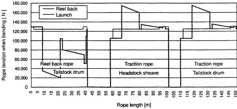
Figure 11: Line pull while bending.
