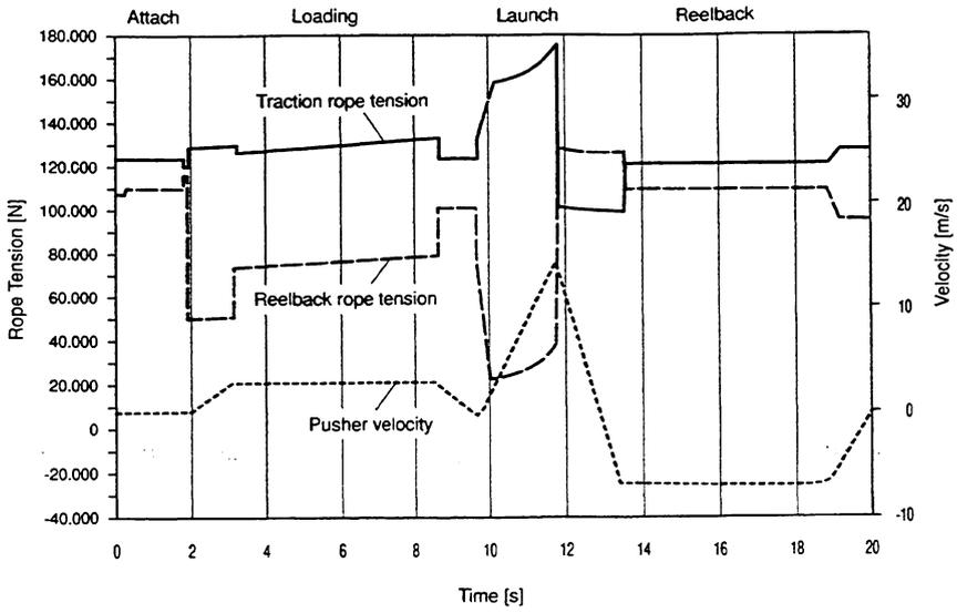
Figure 10: Rope tensions and train velocity over time.
