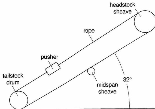
Figure 5: Schematic drawing of the catapult.
