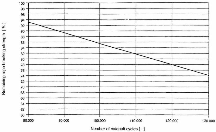
Figure 17: Remaining breaking strength of the rope as a function of the number of catapult cycles.
