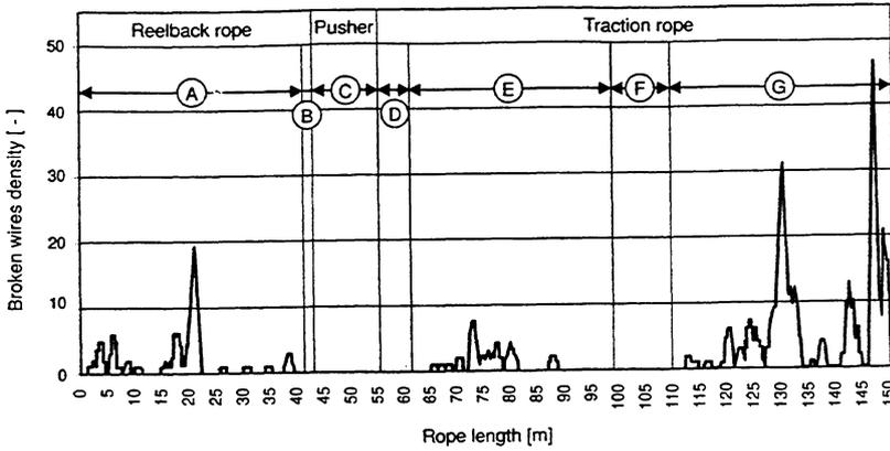
Figure 18: Broken wire density on 30 x d as a function of the rope length.
