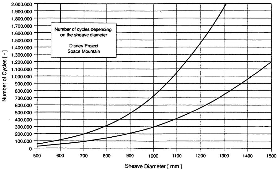
Figure 13: Number of cycles depending on the sheave diameter.
