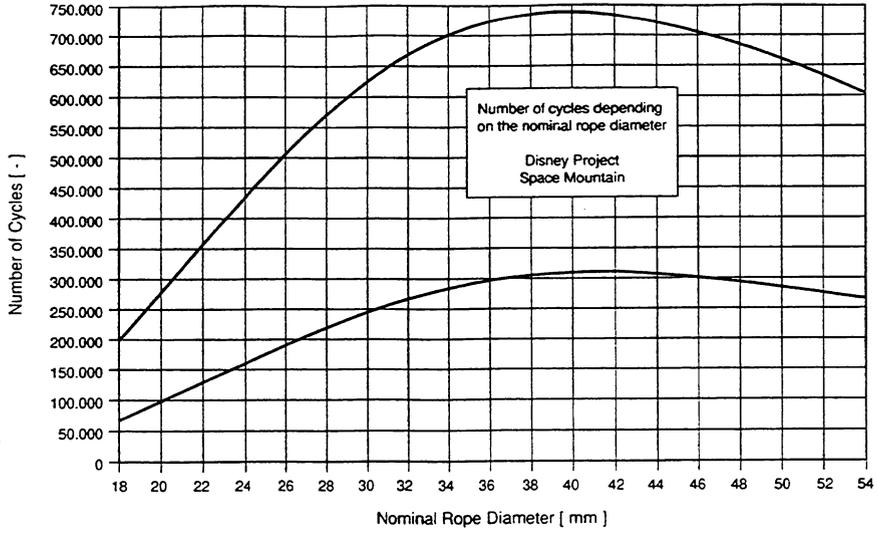
Figure 12: Number of cycles depending on the nominal rope diameter.
