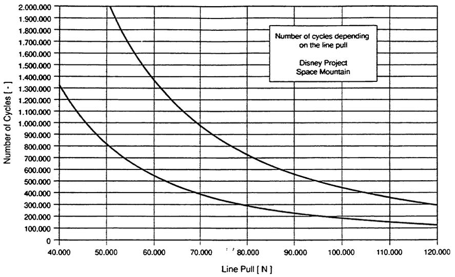
Figure 14: Number of cycles depending on the line pull.
