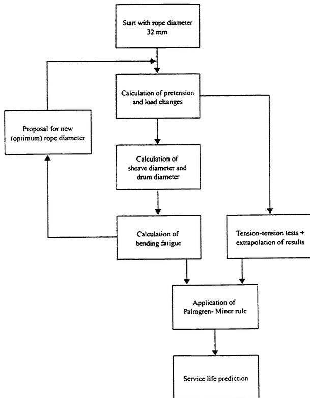
Figure 15: Flow chart showing the calculation procedure
