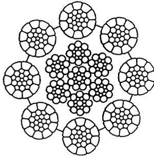
Figure 6: The rope: Casar Turboplast.
