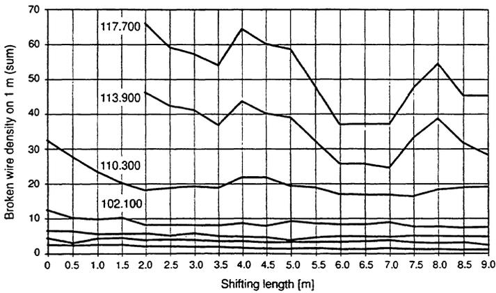
Figure 19: Hypothetical number of wire breaks depending on the shifting length.
